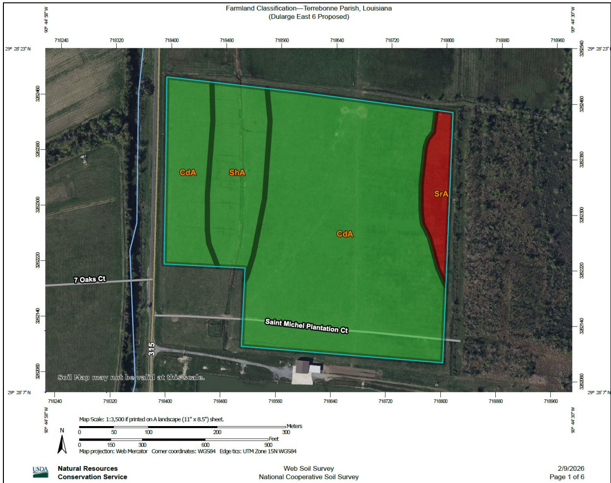
Figure 4. Potential borrow pit for Reach F levee construction, Dularge East - 6. Located in Terrebonne Parish, Louisiana.
